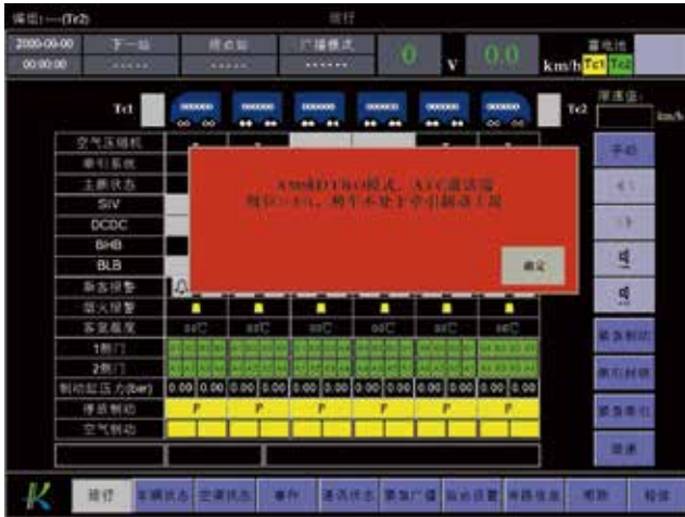
图5 HMI弹窗报警 Fig.5 HMI alarm in pop-up window
