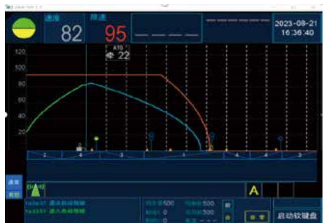
图9 加速至82 km/h后辅助驾驶曲线显示界面 Fig.9 Assisted driving curve display interface after acceleration to 82 km/h
