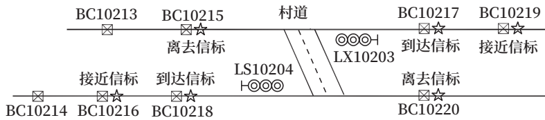
图4 无站台关联的平交路口 Fig.4 Level crossing not associated with the platforms
