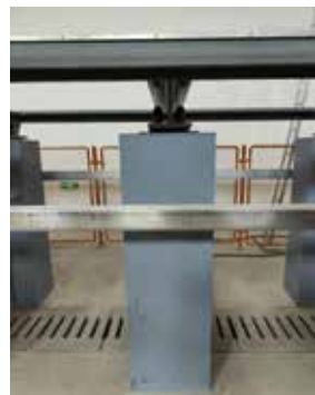
图2 中低速磁悬浮接触轨 Fig.2 Medium and low speed maglev contact rail
