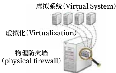
图1 虚拟防火墙逻辑系统 Fig.1 Logical system diagram of virtual firewall
