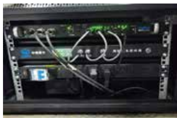
(b) 车载卫星接收机及定位数据记录装置 (b) Vehicle satellite receiver and positioning data recording device
