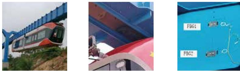
(a)试验线外观图1 (b)试验线外观图2 (c)FBG安装布置
