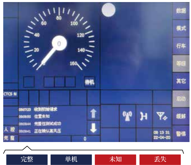
图1 DMI界面完整性状态显示 Fig.1 Display of integrity state on DMI interface
