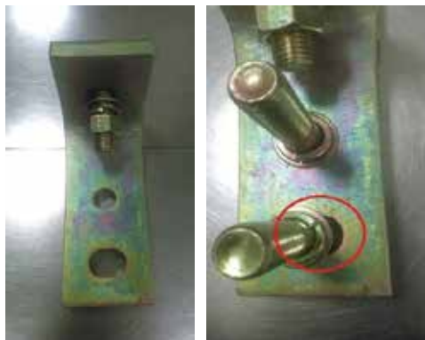
图6 安装螺丝垫圈未完全覆盖 Fig.6 Incomplete covering of screw washer
