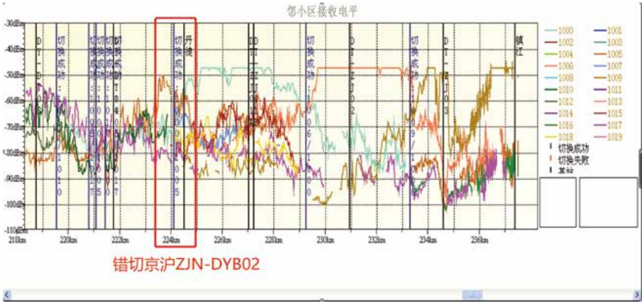
图2 沪宁测试车错切至京沪线ZJN-DYB02基站 Fig.2 Incorrect handover to Base Station ZJN-DYB02 of the Beijing-Shanghai High-speed Railway performed by the test train of the Shanghai-Nanjing Intercity Railway
