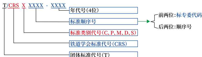
图3 中国铁道学会团体标准编号 Fig.3 Composition of CRS association standard number
