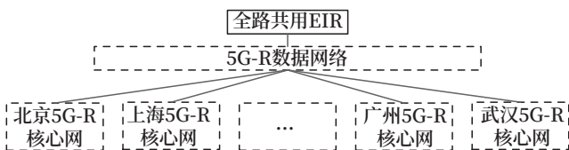
图3 全路共用设置方案示意 Fig.3 Plan for one shared EIR for the entire railway network
